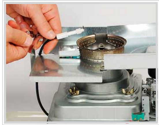
Step 8 Lift off the igniter.
