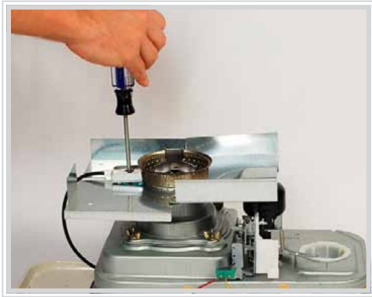
Step 7 Remove the screw.
