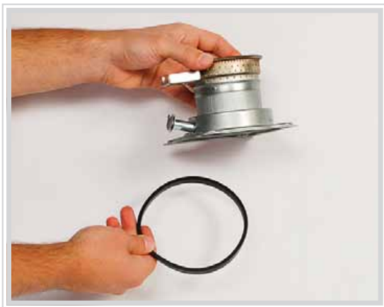
Step 11 Remove the gasket.
