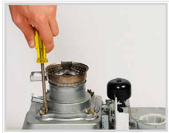
Step 10 Unscrew 4 wing nuts and remove the wick holder assembly.
