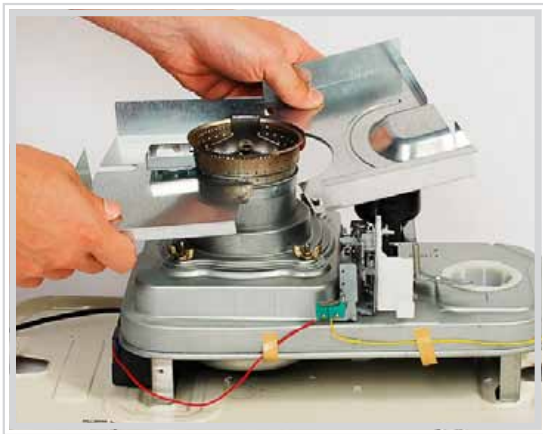
Step 9 Separate the wing cover into 2 pieces. Caution: The edge is very sharp.
