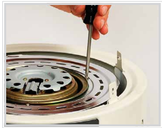
Step 8 Remove 3 screws securing the shelter plate and remove it.
