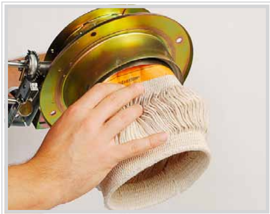
Step 11 To remove the wick from the adjuster, fold it and slide it out. Caution: the teeth holding the wick are very sharp.
