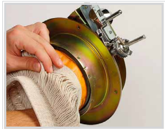
Step 12 The replacement wick has a black line. Fold the new wick and slide it into the adjuster. The black line on the outside of the wick should match the bottom edge of the adjuster. Press the wick against the teeth inside the adjuster to obtain a firm grip. Start at the bottom row of teeth and slowly work your way up in a circular motion.
